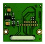
SINTF-ADP-EDT display adapter to connect an EDT display (3.5"-7")
