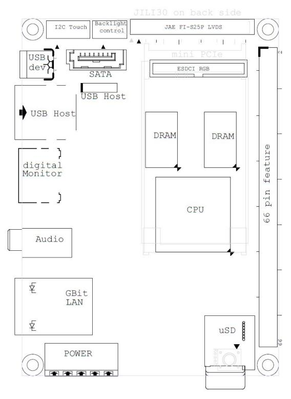
Figure 3: Connector Layout
