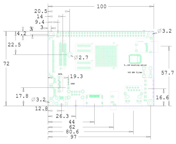
Figure 2: Mechanical Dimension
