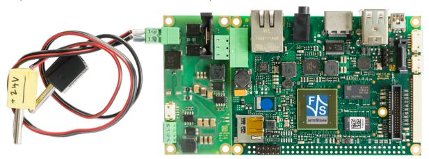
The extension board is designed to plug it into the power Connector of the armStone. For more information check the F&S website:
