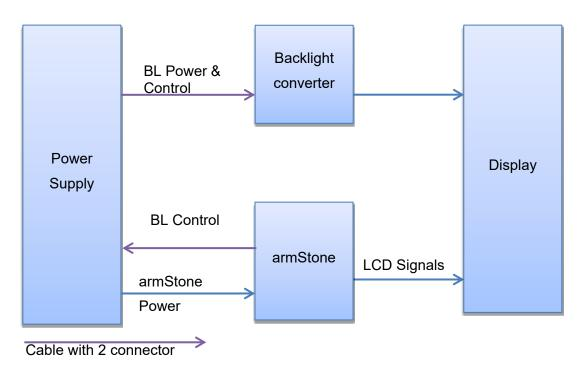
Figure 5: backlight connection with 2 cable
