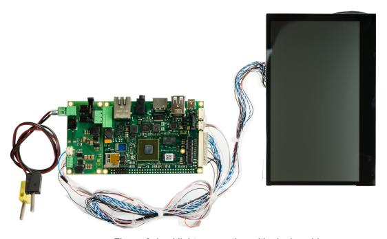
Figure 6: backlight connection with single cable
