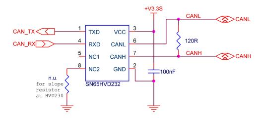
Figure 8: CAN transceiver circuit
