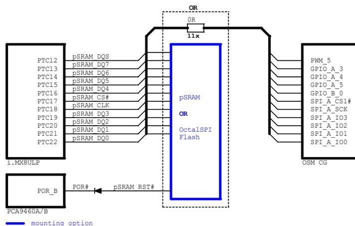
Figure 4: pSRAM / OctalSPI Flash (mounting option)
