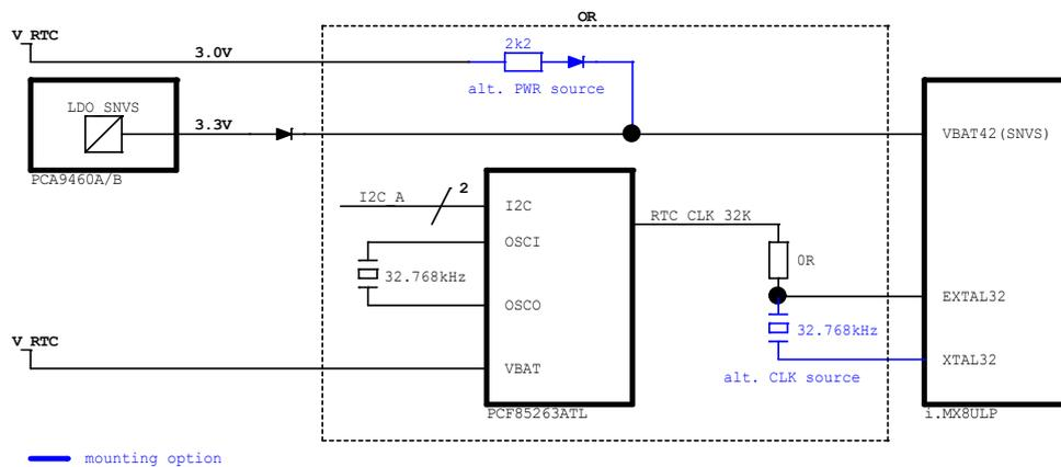
Figure 5: RTC (mounting options)
