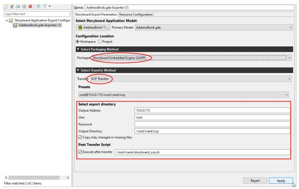
Figure 4: Setup Storyboard Application Export Configurations
