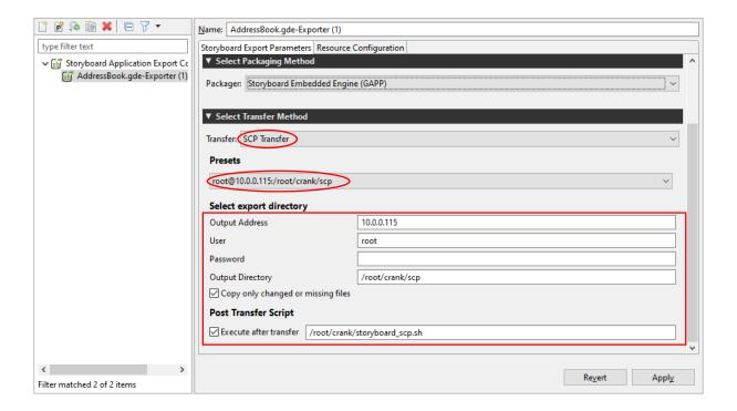
Figure 7: Setup Storyboard Application Export Configurations
