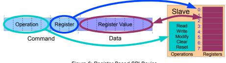
Figure 6: Register Based SPI Device
