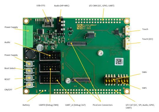
Figure 1: Top side of PicoCoreMX7ULP Starterkit baseboard (PicoCoreBBULP)
