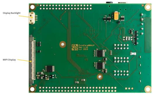
Figure 2: Bottom side of PicoCoreMX7ULP Starterkit baseboard (PicoCoreBBULP)
