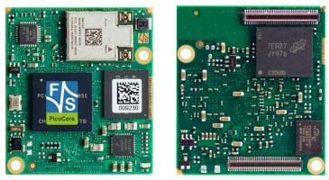
Figure 3: PicoCoreMX7ULP top and bottom view
